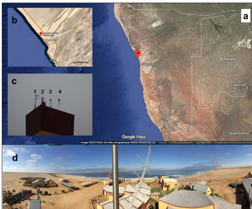
135 Figure 2. Composite of (a) © Google map showing the location of Henties Bay in Namibia, southern Africa; (b) the location of the University of Namibia campus where HBAO was located on the north-west of the town of Henties Bay; (c) some of the sensors and sampling head on the top of the HBAO tower, that is (1) wind sensor; (2) AERONET/Photons sun/sky photometer (3) PM 10 sampling head serving the TEOM and nephelometer instruments; (4) PM 10 sampling head serving the PARTISOL sampler. The PM 1 sampling head serving the aethalometer and the 140 Teflon line serving the ozone analyser are not visible; (d) the view from the top of the HBAO tower to the west, showing the small and few buildings of the University campus and the proximity with the sea shore at approximately than 100 m. The stratocumulus cloud deck is visible at the horizon. Copyright statement: Map data © NASA © 2025 Google.
