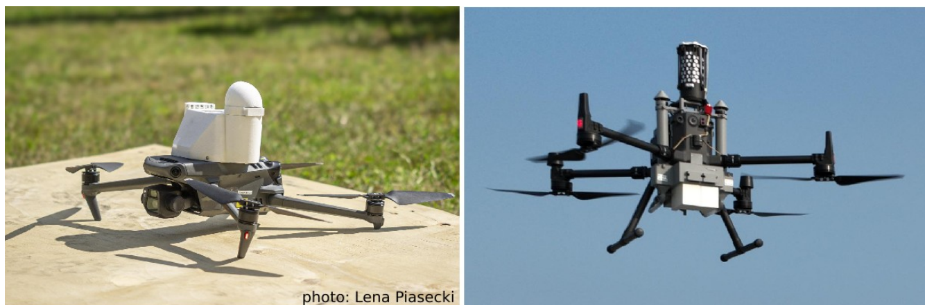
Figure 7. Multicopter “Flik” (left, DJI Mavic 3 Enterprise) and “Hopper” (right, DJI Matrice 300 RTK) with custom PARASITE payloads, both operated by the University of Tübingen. Foto credits: left: Lenu Piasecki, University of Cologne, right: Andreas Platis, University of Tübingen
