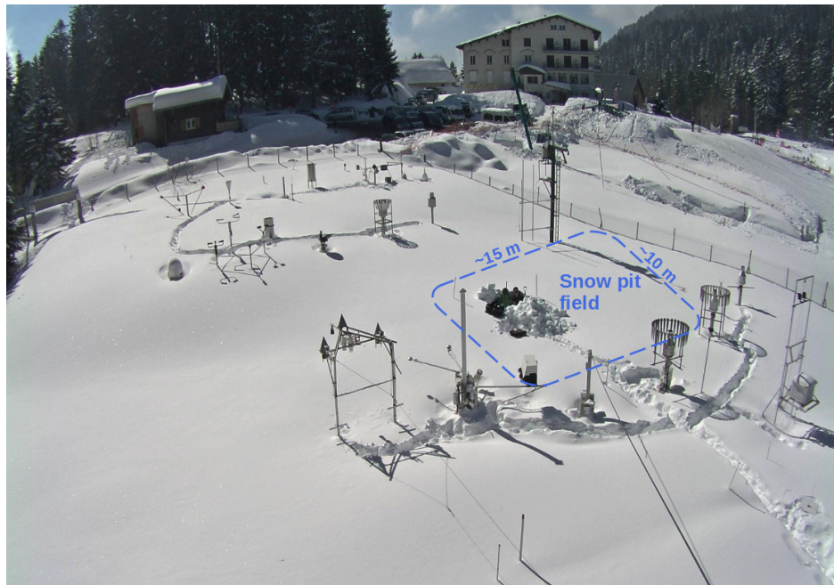
Figure 1. Picture of the observation field site for automatic and manual measurements at Col de Porte (credit: Y. Lejeune, CNRM). The snow pit field, in which the IVORI measurements were done, is shown.
