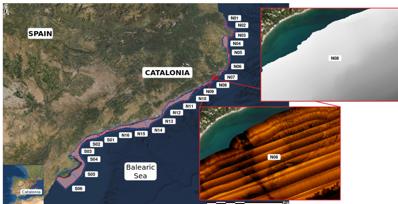
Figure 1. Overview of the surveyed area, divided into 22 sectors, illustrating a portion of the mosaiced SSS transects from sector N08 and the corresponding DEM. The basemap was provided via Esri ArcGIS using OpenStreetMap data. For more information, visit https://www.arcgis.com/home/item.html?id=b834a68d7a484c5fb473d4ba90d35e71 (last access: 15 July 2026).
