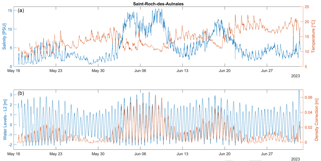
Figure 7. Seametrics CT2X sensor data at Saint-Roch-des-Aulnaies (srda): (a) Salinity and temperature time series; (b) Level-2 water levels with corresponding density corrections.
