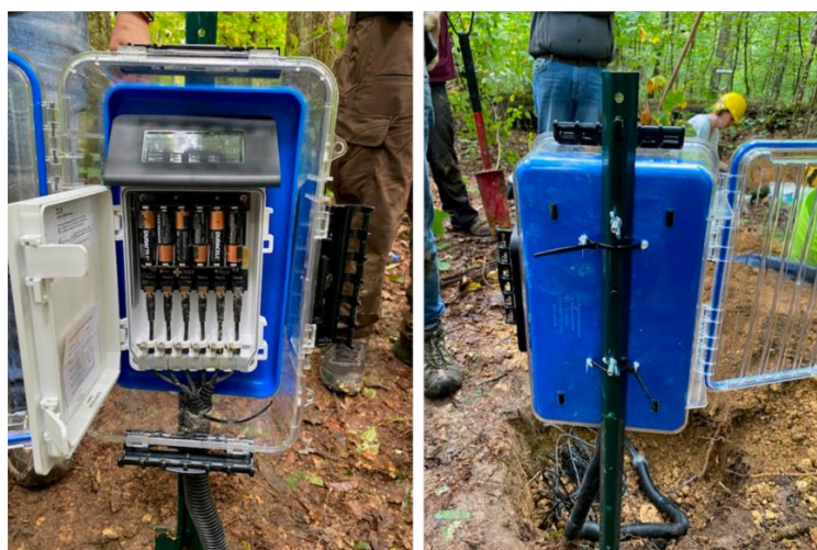
Figure 4. Photographs of a ZL6 data logger installed at the Fernow Experimental Forest. The data logger was encased in a clear tackle box and zip tied to a metal T-post which was driven into the ground. Sensor wires were encased in black split loom tubing and passed through a hole
