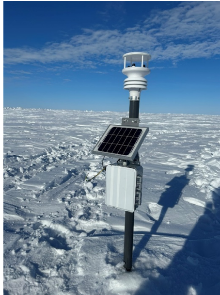
Figure S4: UiT MaxiMet GMX560 micro-met station deployed at the same ice floe as the SIMB3_2024K ice mass balance buoy.
