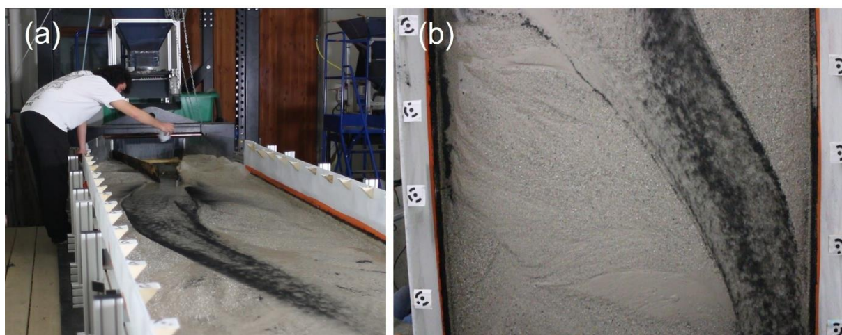
315 Figure 11: (a) Example of tracers spreading in the channel. (b) Top view as shown in the LSPIV videos.
