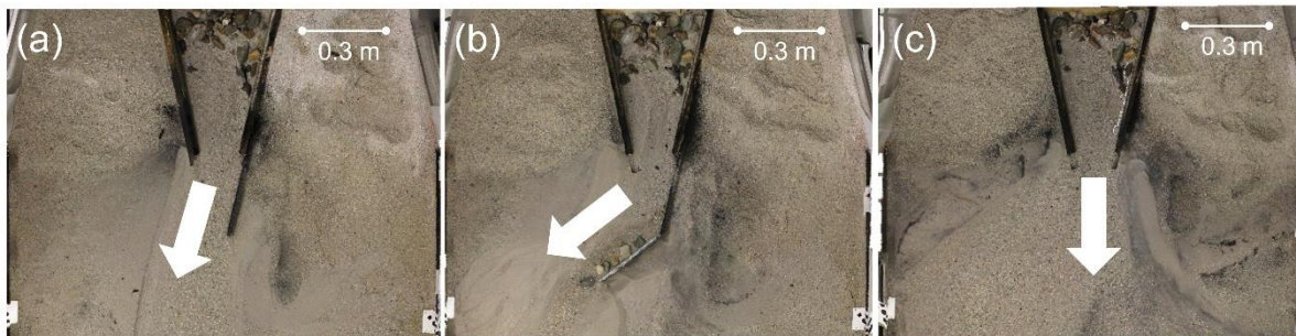
115 Figure 3: The different upstream inflow configurations: (a) 12° (configuration 1), (b) 52° (configuration 2), and (c) 0° (configuration 3).
