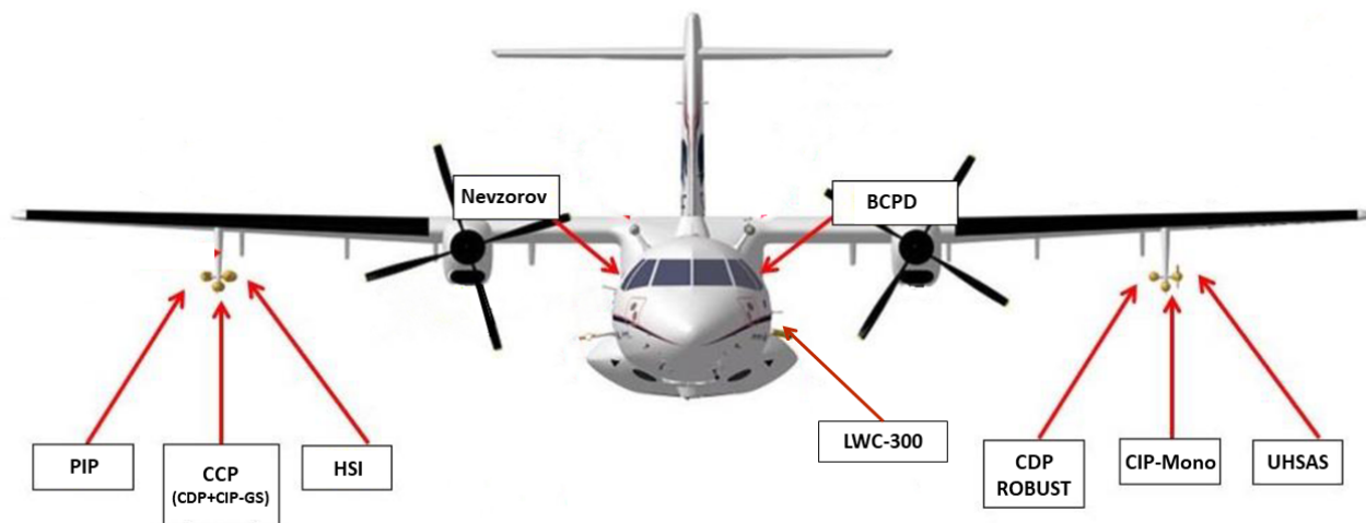
Figure 3. Location of cloud instruments on the ATR 42. In total, the aircraft carried 6 underwing cloud probes and 2 fuselage-mounted instruments.
