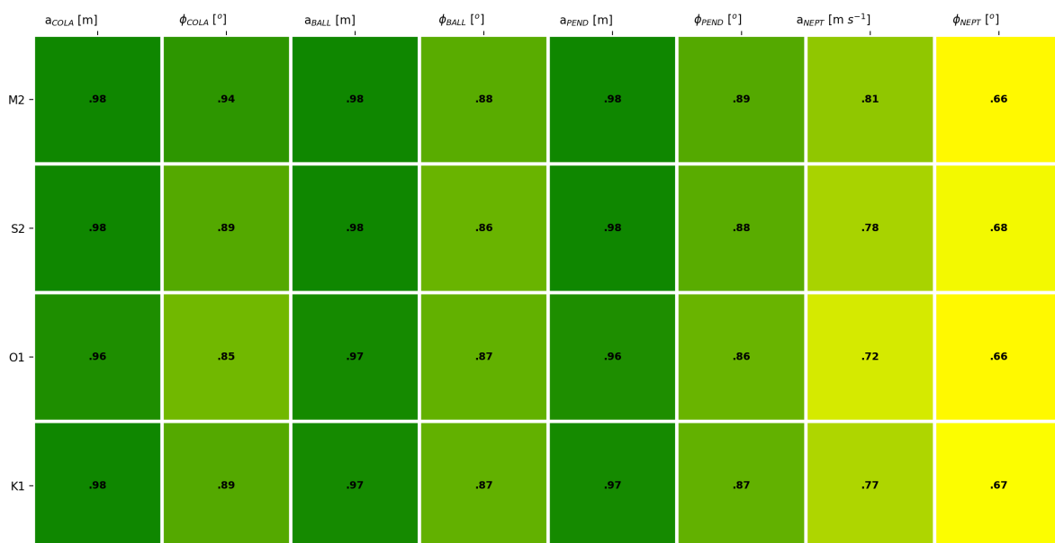
Figure 5. Correlation coefficient ( R^2 ) of the M2, S2, O1 and K1 constituents of water level and currents for Cola, Pendulo and Ball stations, and Neptune station, respectively. The color indicates the degree of accuracy (green indicates excellent agreement, yellow-orange indicates good agreement, and red indicates poor agreement).
