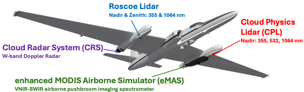
685 Figure 1: Schematic that shows the physical location of the CPL, Roscoe, CRS, and eMAS sensors on the NASA ER-2. This schematic was created by annotating a NASA Airborne Science Program 3D model of the ER-2 ( https://airbornescience.nasa.gov/3d-models/ ).
