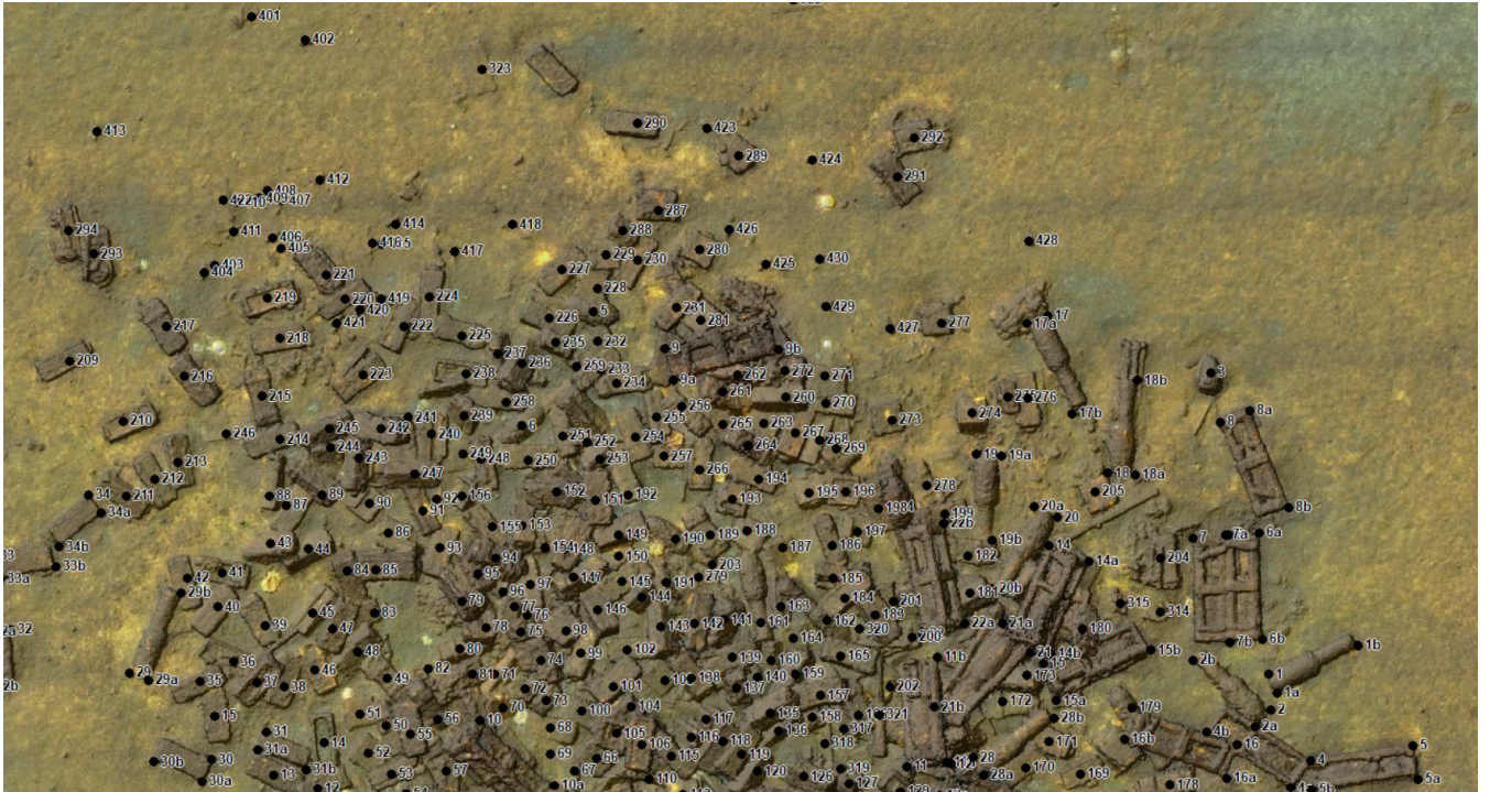
Figure 2. Example part of an annotated photomosaic. The figure shows the northern half of munition pile Haf_00318 as annotated by expert 1. Numbers with lowercase letters indicate objects that were measured in 2 dimensions (e.g., objects 1 and 8 in the east). The expert counted 483 objects and measured 52 of them, with the largest one measuring 1.24 m in length. (© 2026 DSM, GEOMAR)
