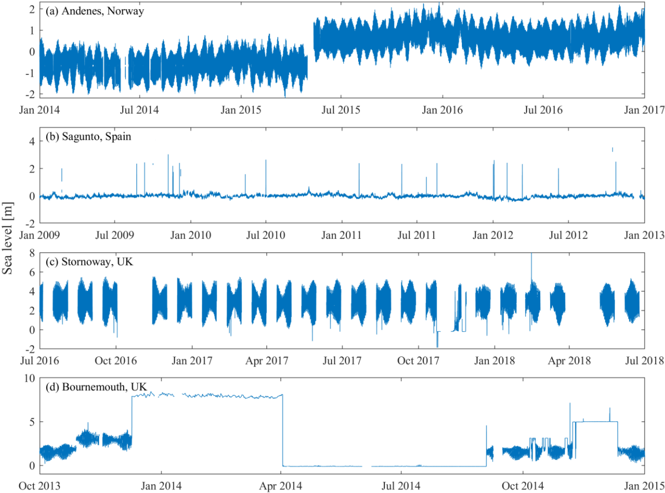
Figure 2. Examples of errors commonly encountered in raw sea level time series: (a) vertical shifts; (b) spikes; (c) gaps and spikes; (d) spurious data, flat lines, and clustered spikes.
