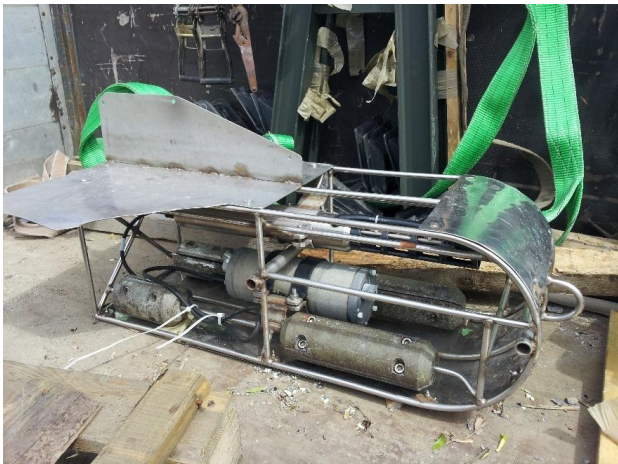
111 Figure 2: CTD towed probe system used for the collection of data with Sea-Bird SBE49 (2002-2020)
