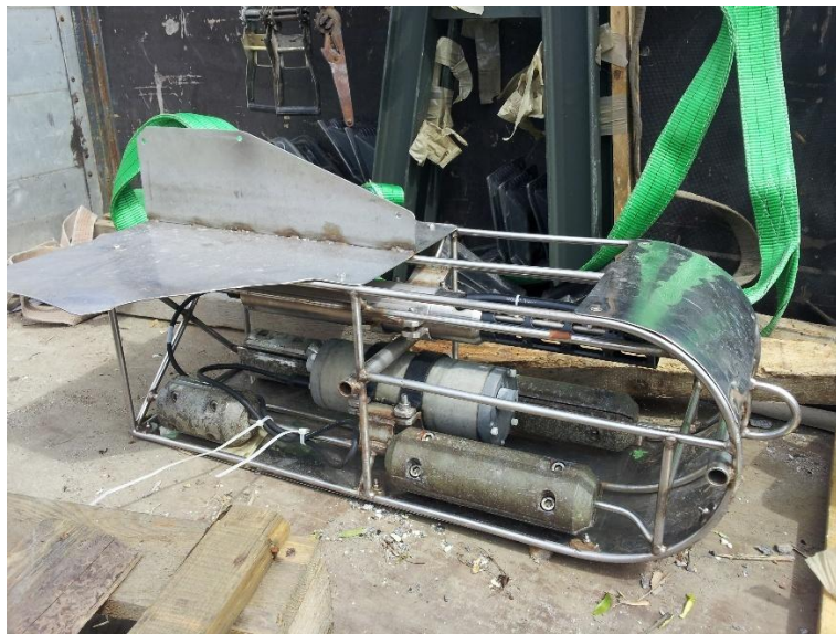
Figure 2: CTD towed probe system used for the collection of data with Sea-Bird SBE49 (2002-2020)
