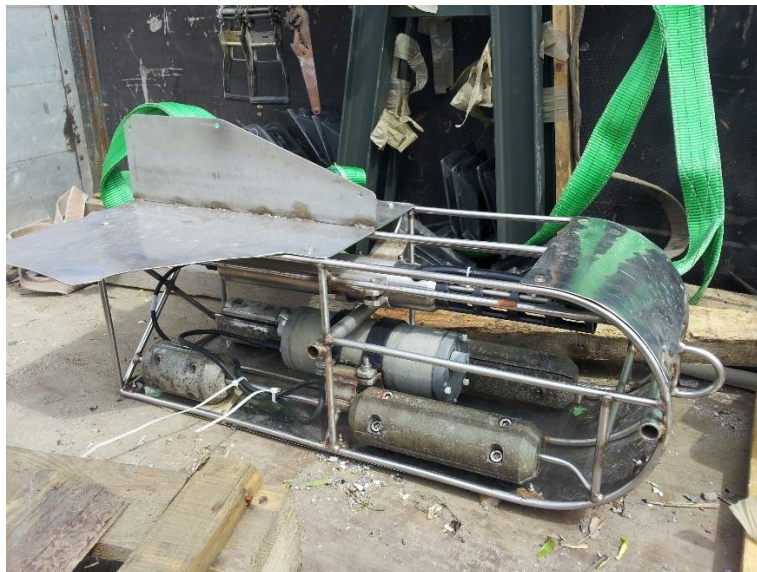
144 Figure 2: CTD towed probe system used for the collection of data with Sea-Bird SBE49 (2002-2020)
