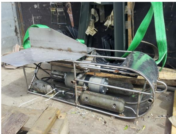
144 145 Figure 2: CTD towed probe system used for the collection of data with Sea-Bird SBE49 (2002-2020)
