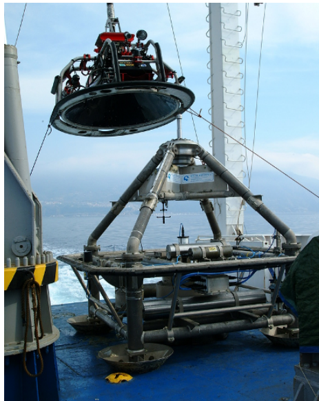
Figure 1: Example of a GEOSTAR-type observatory integrating multidisciplinary sensors. The image shows the NEMO-SN1 benthic observatory during the GNDT-1 campaign (2002–2003).
