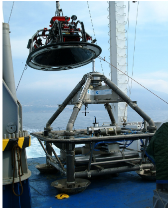
Figure 1: Example of a GEOSTAR-type observatory integrating multidisciplinary sensors. The image shows the NEMO-SN1 benthic observatory during the GNDT-1 campaign (2002–2003).
