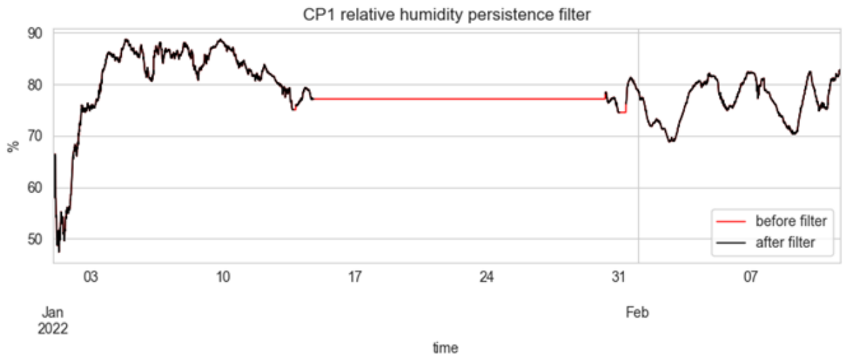
Figure 10. Illustration of how the persistence filter operates. The filter identifies sequences of measurements that remain unrealistically constant over time. Values showing no expected natural variability within a specified window are flagged as potential sensor malfunctions or data artifacts.
