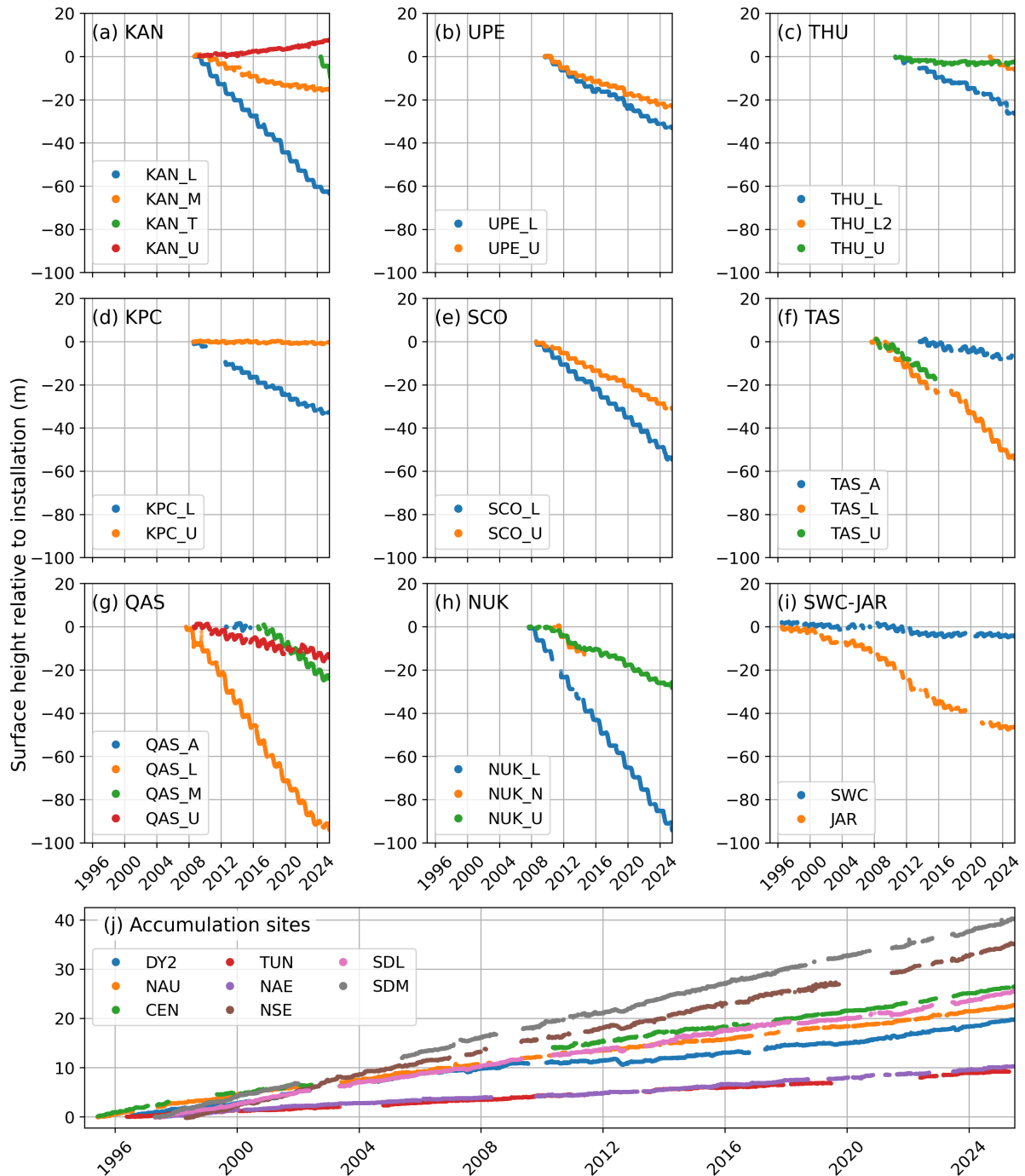
Figure 13. The integrated surface-height product ( z_{surf\_combined} ) for all PROMICE and GC-NET sites. This variable merges observations from sonic rangefinders, pressure transducers, and stake-mounted sensors to produce a continuous elevation record that also supports estimates of time-varying thermistor depths.
