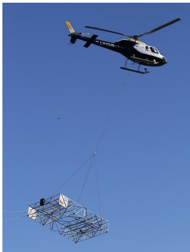
Figure 2 Picture shows the 25 MHz antenna of the FAU attached to a Eurocopter AS355 Écureuil 2
