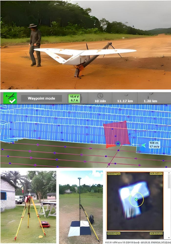
565 Figure 13: UAV-LS acquisitions at FBRMS-02: Lopé using a fixed-wing system. This UAV employs a conventional take-off 566 and landing (CTOL) procedure, with launch aided by a catapult. Once airborne, the UAV is controlled from a laptop connected
