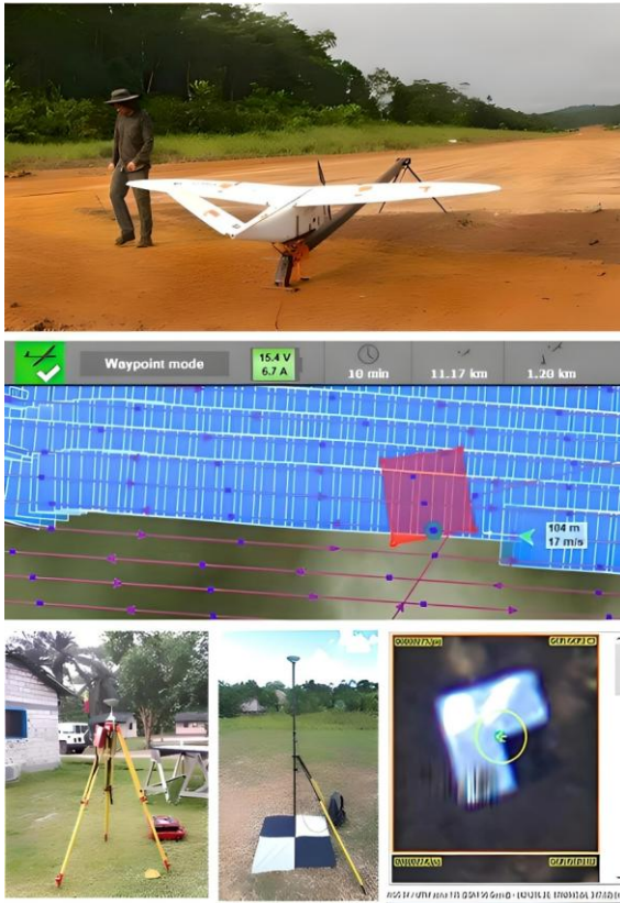
Figure 11: UAV-LS acquisitions at FBRMS-02: Lopé using a fixed-wing system. This UAV employs a conventional take-off and landing (CTOL) procedure, with launch aided by a catapult (top). Once airborne, the UAV is controlled from a laptop connected to the UAV via an antenna (middle). The flight trajectory is corrected to centimetre precision using data collected from a static GNSS receiver placed within 10 km of the UAV operating area (lower left). Additional refinements and corrections are possible via ground control points located across the study area (lower middle), the positions of which are measured using a ‘rover’ GNSS receiver (lower right). Image originally published in McNicol et al. (2021).
