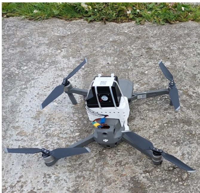
Figure 1. The DJI Mavic 2 pro equipped with a drone air quality backpack.
