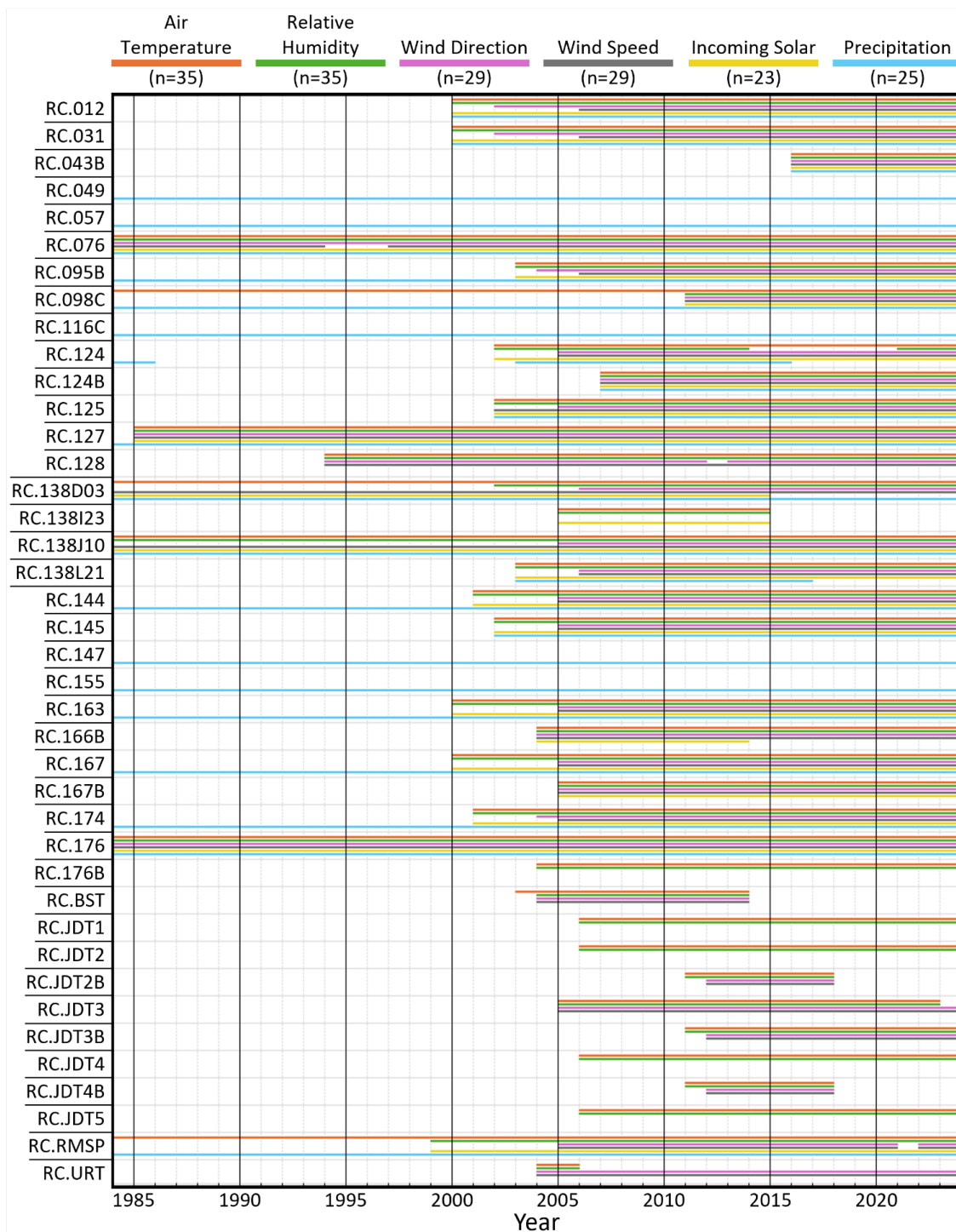
95 Figure 3 – Measurement record from the 40 individual sites within RCEW for the time-period October 1, 1983 - September 30, 2023. Some sites measure all six variables needed by the Spatial Modeling Resources Framework to produce the twelve gridded hydrometeorological forcing variables, though many are instrumented to measure fewer variables. Five stations solely measure precipitation alone (RC.049, RC.057, RC.116C, RC.147, and RC.155).
