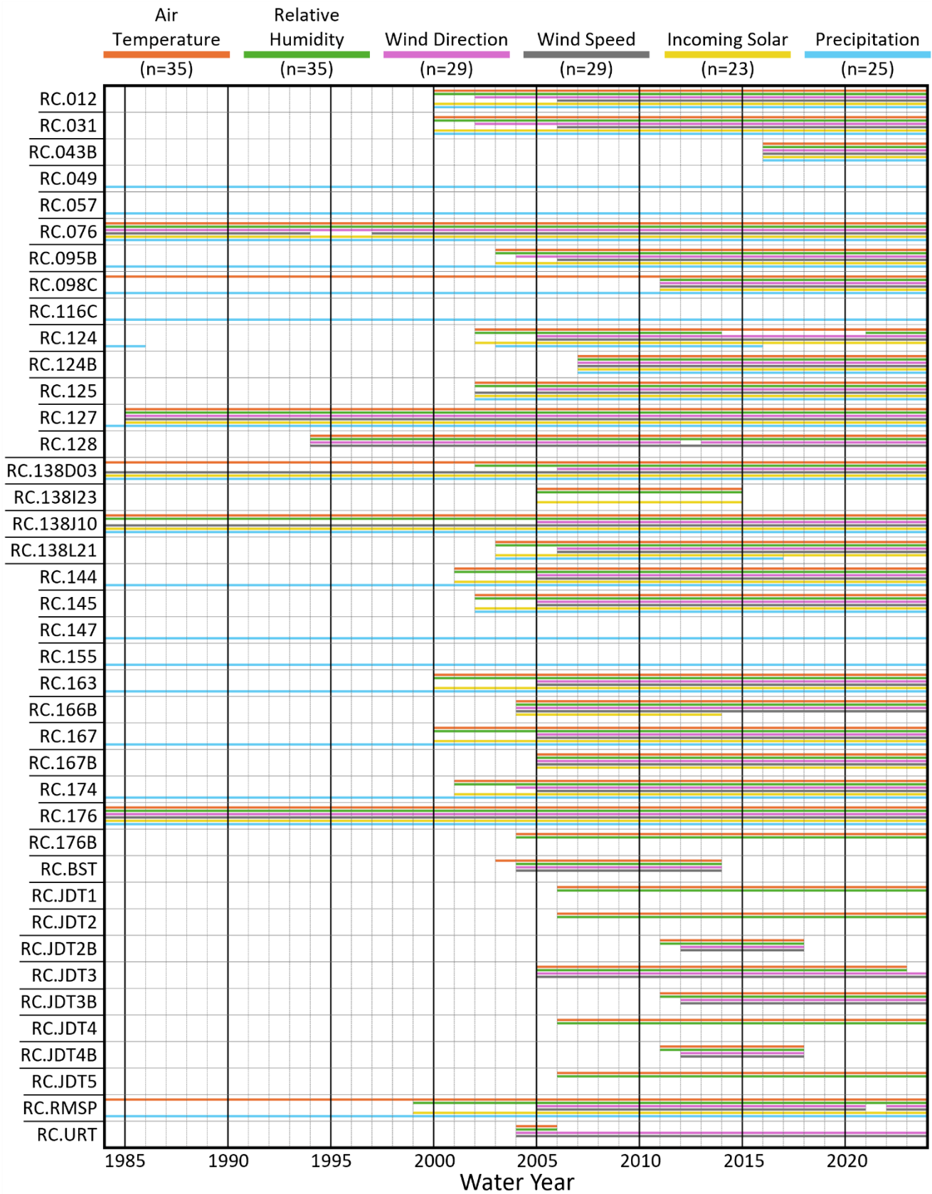
Figure 3 – Annual water year measurement record used in SMRF gridded interpolation from the 40 individual sites within RCEW from 1 October 1983 to 30 September 2023. The horizontal bars for each variable indicate station observation data present for over half of a water year, however smaller data gaps are not shown. Some sites measure all six variables required by
