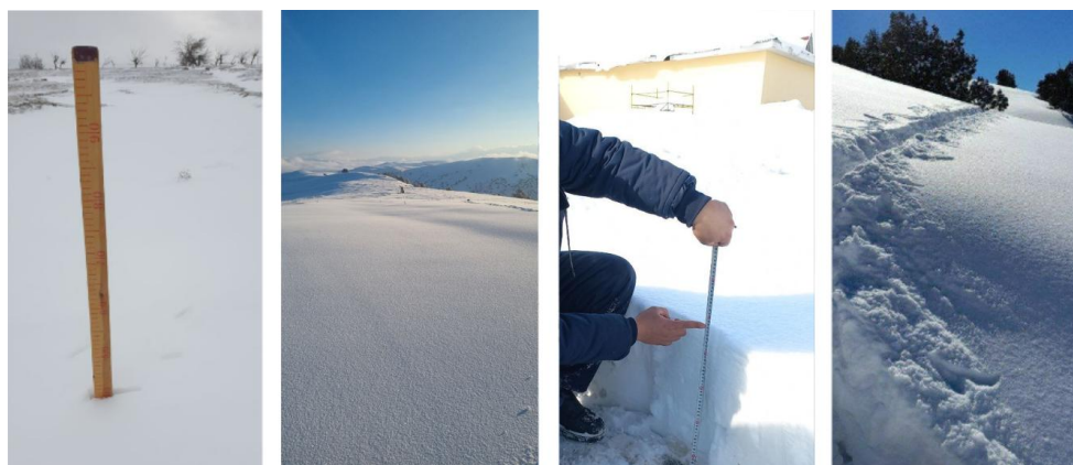
Figure 2. Images sent by volunteers displaying the snow depth measuring process. Used with permission from Erkin Abdulhatov, UZB-METEO group administrator.
