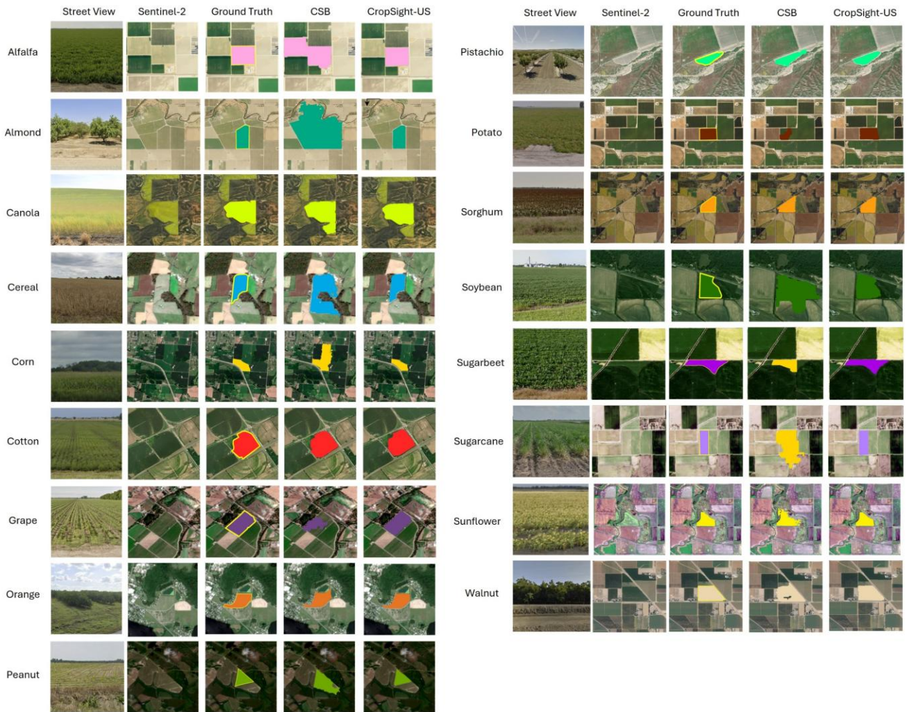
600 Figure 10: Examples across the 17 crop types showcasing roadside field-view GSV imagery, corresponding Sentinel-2 satellite imagery, object-based crop type ground truth, and object-based crop type information generated by Crop Sequence Boundary (CSB) and our ground-truthing framework developed to produce the CropSight-US dataset. GSV images are from © Google Maps, and Sentinel-2 imagery thumbnails are from © European Union/ESA/Copernicus, processed via Google Earth Engine.
