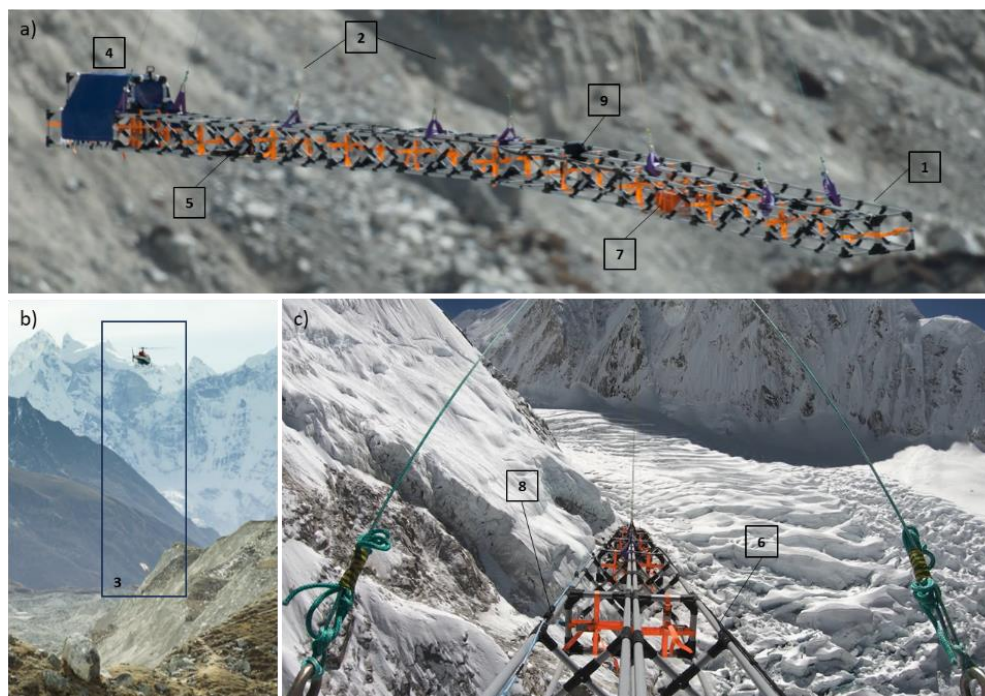
Figure 1 | The radar frame consisting of lightweight fibreglass modules strapped together (1), with rope lines (2) to suspend the system under the helicopter (3), a tail (4) to prevent ‘weathercocking’, a pulse transmitter (5) and corresponding, resistively loaded transmit dipole antenna (6), receiver (7) and receive antenna (8) and GPS (9) (Pritchard, King et al. 2020). Panel (c) shows the system approaching the icefall on Khumbu Glacier (Figure 2), with multiple potential sources of radar clutter notably from the surrounding mountains and crevasse walls. Photo credits: Hamish Pritchard.
