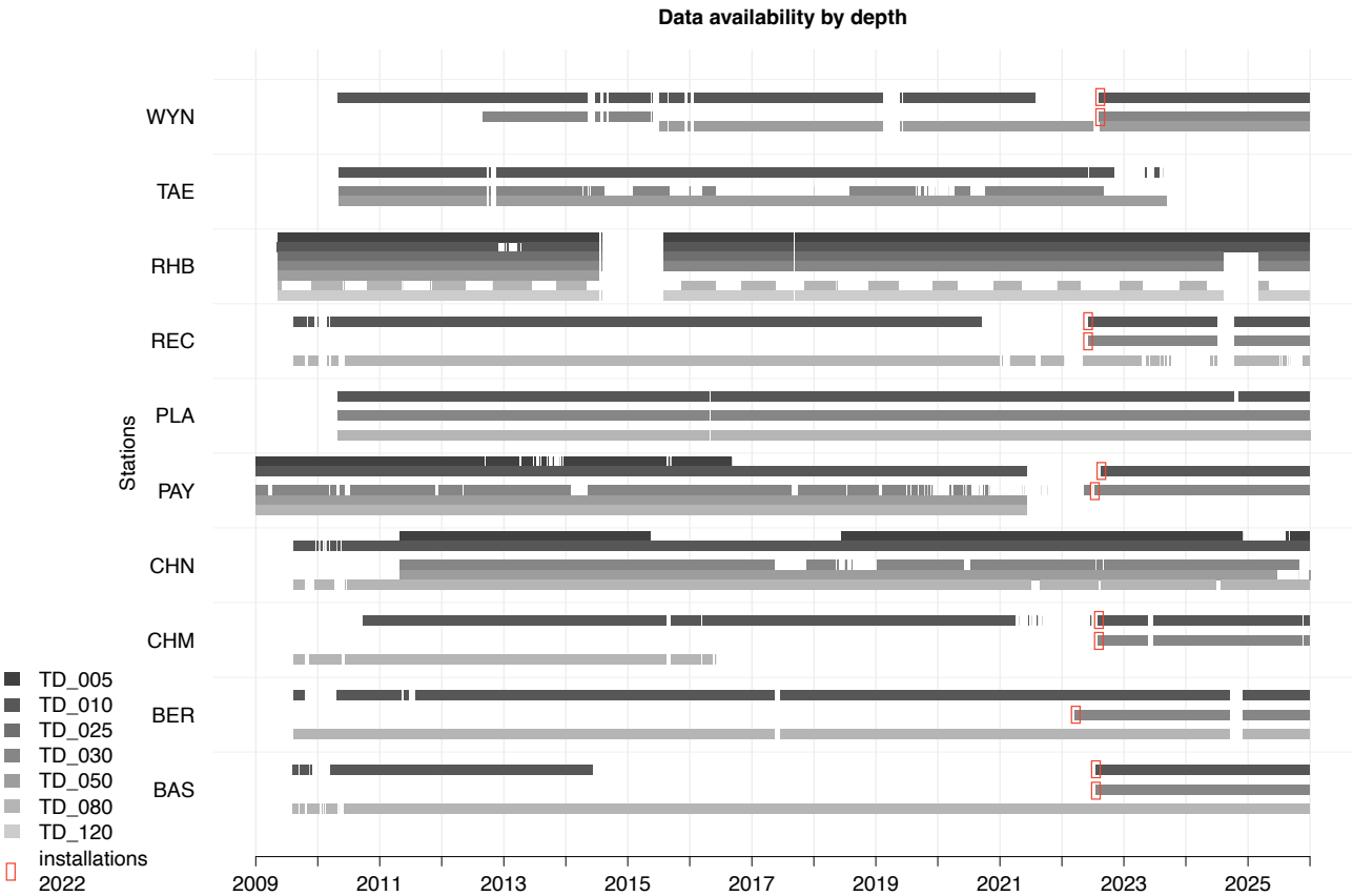
Figure 2 Time series diagram of the IMKO TRIME-PICO TDR (TD) sensor availability at the SwissSMEX grassland stations on the Swiss Plateau. Abbreviations for station names are given in Table 1; numbers alongside the sensor type indicate the installation depth in cm. This is a condensed view that combines all redundant sensor profiles. Note that station RHB includes an additional sensor at 25 cm depth, and that the sensors at the other depths are partly shifted by 5 cm in this profile. For simplicity, the sensors installed at depths of 15 cm, 35 cm, and 55 cm are shown as TD_010, TD_030, and TD_050, respectively. The TDR installations in 2022 are highlighted by red rectangles.
