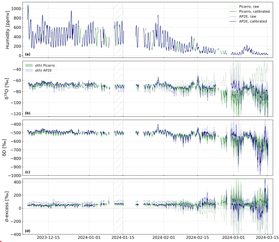
Figure 6: Time series (December 6th 2023 to March 15th 2024) of the atmospheric humidity (in ppmv, panel (a)), \delta^{18}\text{O} (in ‰, panel (b)), \delta\text{D} (in ‰, panel (c)) and d-excess (in ‰, panel (d)) measured by the Picarro (green lines) and AP2E (blue lines) analysers. In panels (b), (c) and (d), the green and blue shaded areas correspond respectively to \sigma(h) (Sect. 2.2.4) of the Picarro and AP2E analysers. In all four panels, the dashed lines correspond to the raw data given by the spectrometers and the plain lines correspond to the corrected and calibrated data (see Sect. 2.2 and 3.1). The grey hatched area marks the period from January 11th to January 15th shown in Fig. 7.
