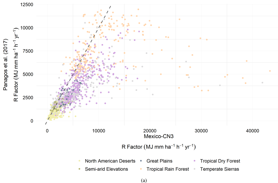
Figure 9. Scatter plot of R factor values from the global rainfall erosivity surface from Panagos et al. (2017) and the R factor estimated with the Richardson et al. (1983) power law equation with the rainfall time series of the Mexico-CN3 (1988-2017) database.
