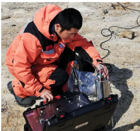
Figure S1. Pictures of collecting ambient air sample using a sampler and canister at Swan Ridge, Zhongshan Station.
