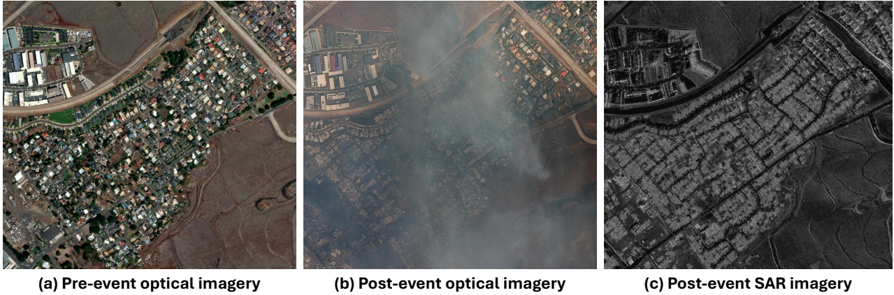
Figure 1. An example of the wildfire occurring in Maui, Hawaii, USA, August 2023. (a) Pre-event optical imagery (© Maxar). (b) Post-event optical image (© Maxar) with land-cover features obscured by wildfire smoke. (c) Post-event SAR imagery (© Capella Space) unaffected by smoke, showing the disaster area.
