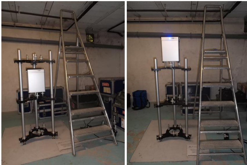
Figure 4: Procedure adopted at Brest for determining the local gravity gradient (top). Illustration of the procedure at mid and top locations using a CG5 relative gravimeter above Ref02 floor mark in 2022 (bottom).
