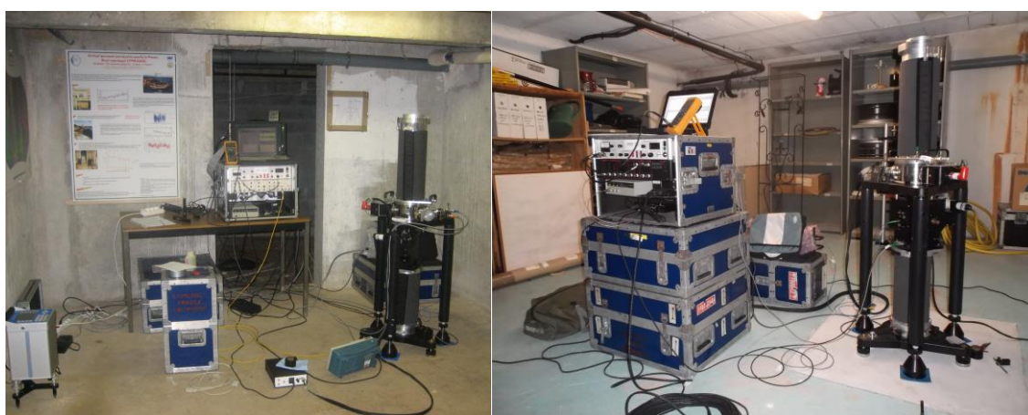
Figure 2: FG5#228 absolute gravimeter observing at Shom in Brest (France) above Ref01 ground floor marker in August 2007 (left) and above Ref02 marker in July 2022 (right).
