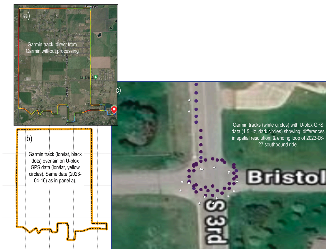
Figure 3: GPS data recorded on Fowler loop ride (2023-04-16) and at termination of southbound Bozeman ride (2023-06-27). Track in panel 'a' came directly from a screenshot of Garmin cyclometer data, with no processing or export. Data in panels 'b' and 'c' came from .csv files relevant to same date, with Garmin cyclometer data exported and converted via .tcx format to .csv while u-blox ZED F9P GPS location and time data (collected at fixed 1.5 Hz recording frequency) came directly from sensor box .csv files. U-blox GPS successfully recorded lane and loop positions at better than 2 m uncertainties during this ride. Users can easily access any sensor data layered on user-selected background in QGIS or other GIS software. Background in panel 'c' came from Google satellite image toggled through QGIS; slight offset occurred due to minor mis-registration. @Google Earth 2023.
