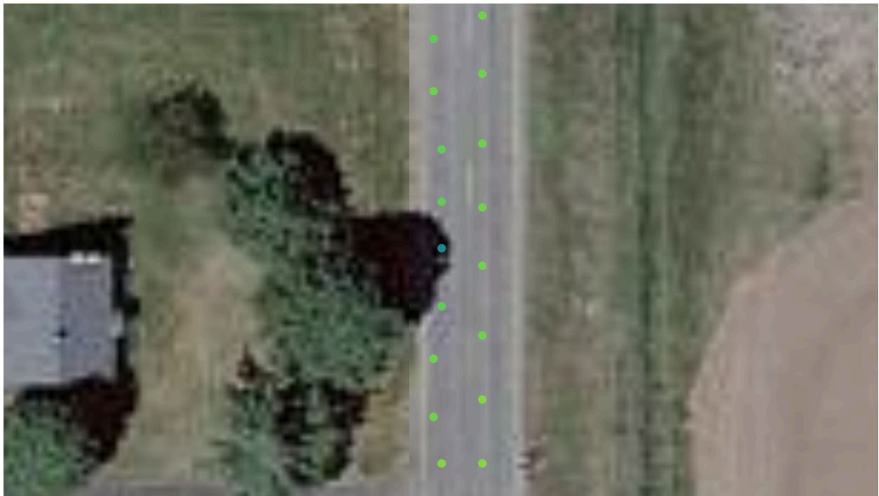
Figure 18: Data from CW and CCW Fowler loop rides on 30 June 2022, demonstrating shade-induced cool surface temperatures measured during CW loop (left track along west lane) followed (less than 20 minutes later) by identical but non-shaded measurements during CCW loop (right track along east lane). Image based on identical temperature scales northbound and southbound. Data clearly demonstrate cooling impact extending part-way across road surface during southbound pass while northbound pass - without shade - shows no impact. (Particular Google Earth image as GIS background, recorded under very similar late-day insolation conditions, tends to emphasize this pattern.) Background data @Google Earth 2023.
