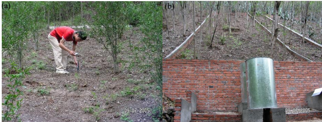
Figure 15. Photos of runoff plot: (a) agricultural land runoff plot and (b) forest land runoff plot
