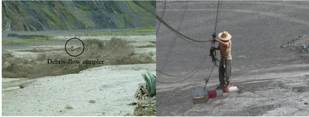
Figure 9. Details of debris-flow sampling.
