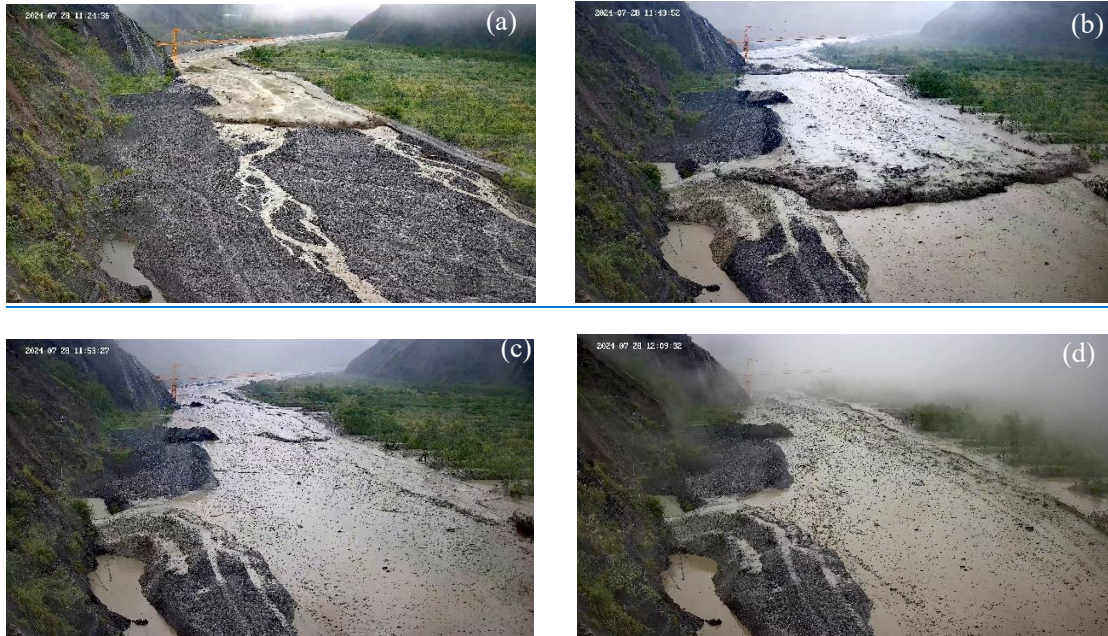
Figure 11. Debris-flow video frames captured on July 28th, 2024: (a) first debris flow surge on coarse bed, (b) surge flow, (c) continuative flow and (d) hyperconcentrated flow.
