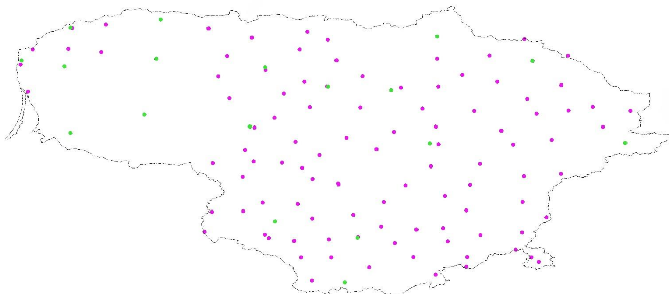
Figure 2: Distribution of the second and third order gravimetric stations (green dots – second order stations; magenta dots – third order stations).
