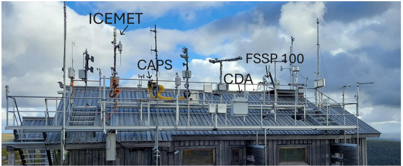
165 Figure 1. The ICEMET, the CAPS, the CDA and the FSSP-100 as they were installed on the roof at the Sammaltunturi site 170 during PaCE 2022.
