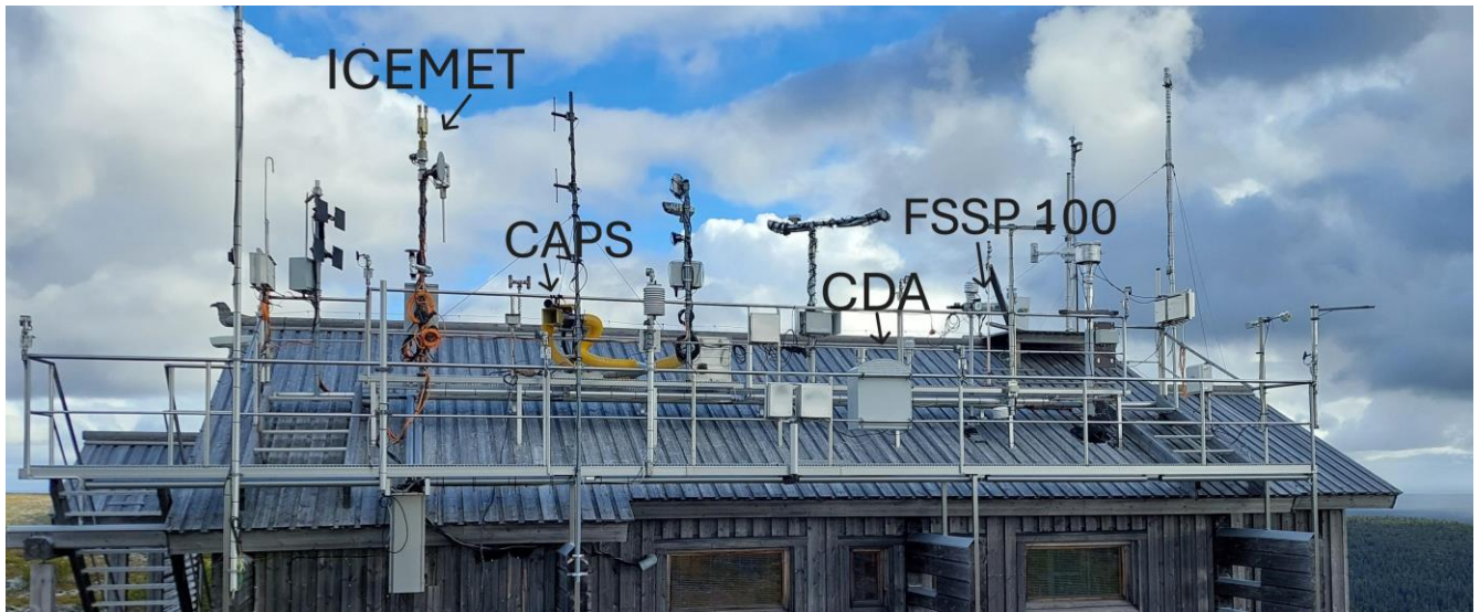
175 Figure 1. The ICEMET, the CAPS, the CDA and the FSSP-100 as they were installed on the roof at the Sammaltunturi site during PaCE 2022.
