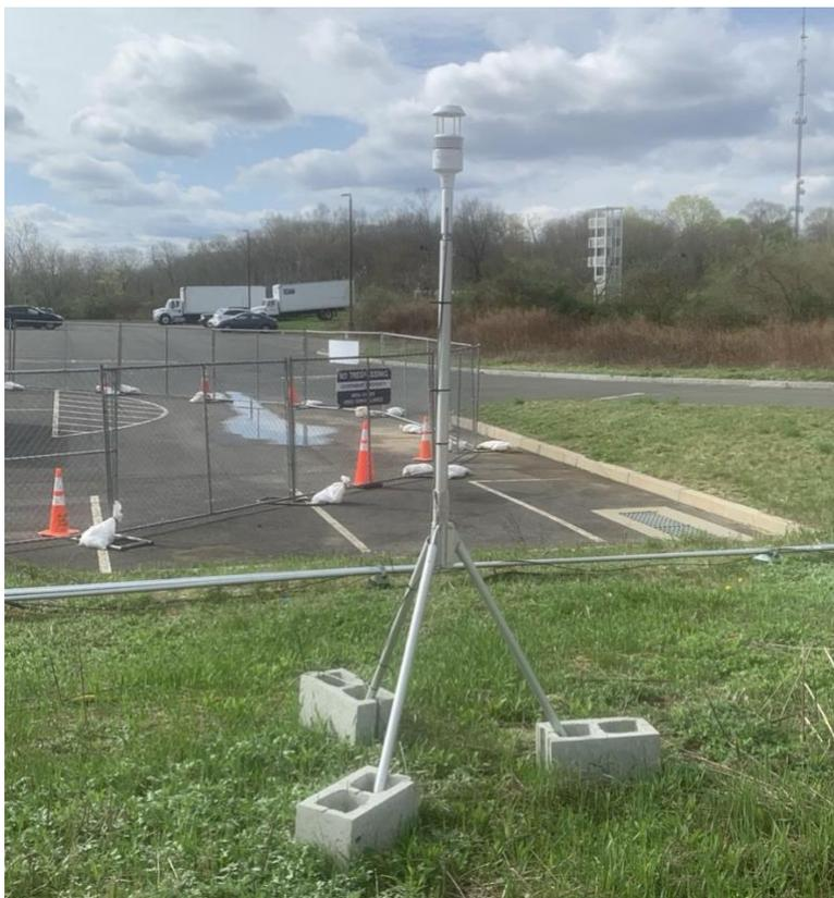
155 **Fig. 2. Deployment of the Met One All-in-one 2 during 2022-2023 at the D3R site.**
