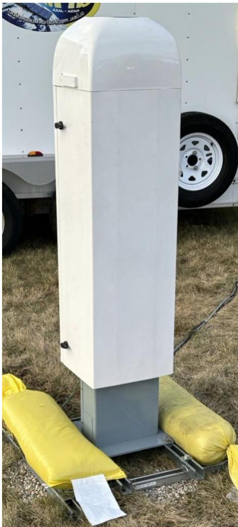
340 **Fig. 12.** Deployment of the Vaisala Ceilometer during 2023-2024 at the GAIL Site.
