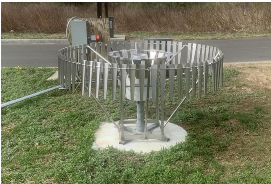
Fig. 4. Deployment of the Ott Pluvio<sup>2</sup> Weighing Gauge during 2022–2023 at the D3R site.
