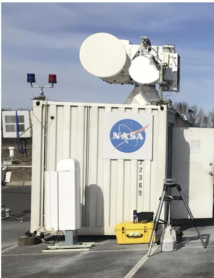
260 **Fig. 7.** Deployment of the ACHIVE trailer with the W-Band Radar on the roof during 2022-2023 at the D3R site.
