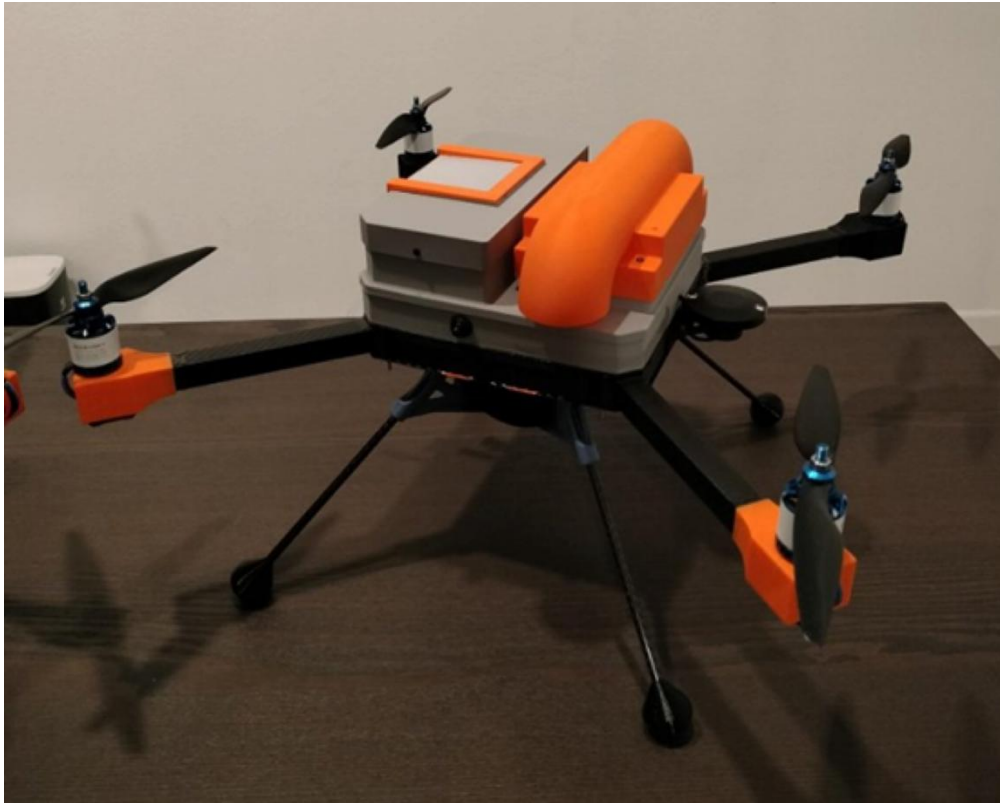
Fig. 11. The Oklahoma StormTrooper: an Unmanned Aerial Weather Measurement System (WxUAS) with its remote (left) and in situ (right) payloads. Deployed during 2023-2024 at the GAIL site.
