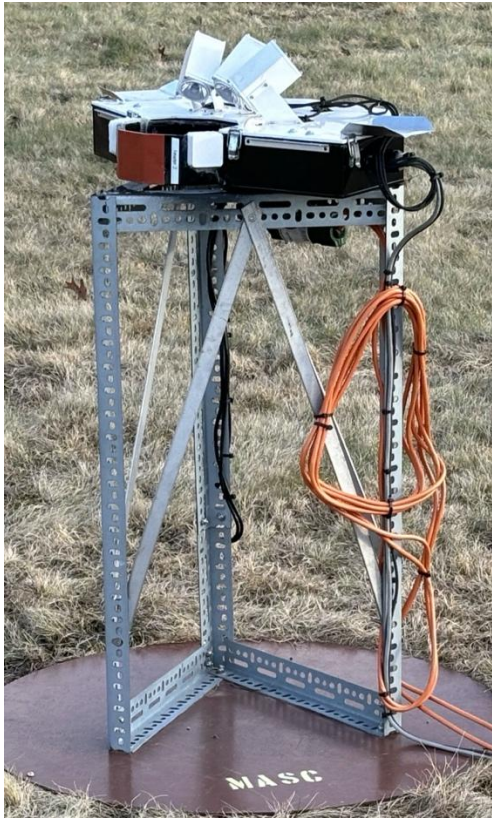
Fig. 10. Deployment of the Multi-Angle Snowflake Camera during 2023-2024 at the GAIL site.
