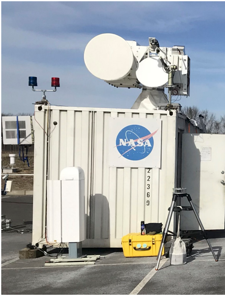
Fig. 7. Deployment of the ACHIEVE trailer with the W-Band Radar on the roof during 2022-2023 at the D3R site.
