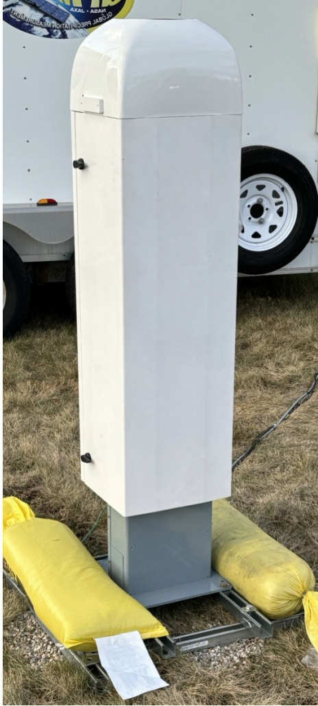
Fig. 12. Deployment of the Vaisala Ceilometer during 2023-2024 at the GAIL Site.
