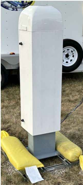
355 Fig. 12. Deployment of the Vaisala Ceilometer during 2023-2024 at the GAIL Site.
