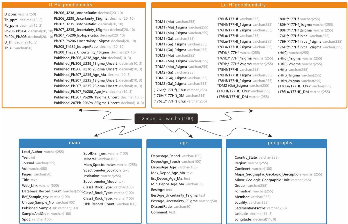
620 Figure 2: Schematic of the OneDZ relational schema. The three core tables (blue) and two geochemical tables are linked by the primary key zircon_id (varchar 100). Black underlines indicate primary keys; arrows denote foreign-key relationships.
