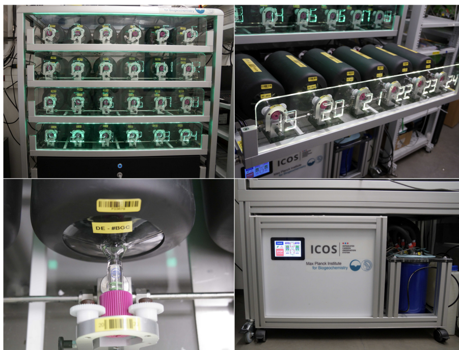
Figure 1. Automated flask sampler installed at the ATTO site. The sampler consists of four trays, and each tray holds six flasks, for a total of 24 flasks available for sampling. A drawer below the last tray contains all the electronic components and the compressor pump. The flasks are of 3 liter volume and samples are stored at an overpressure of \sim 0.7 bar. A drying unit (bottom right) takes the air drawn in by the sampler and cools it to a dew point below -38^{\circ}\text{C} .
