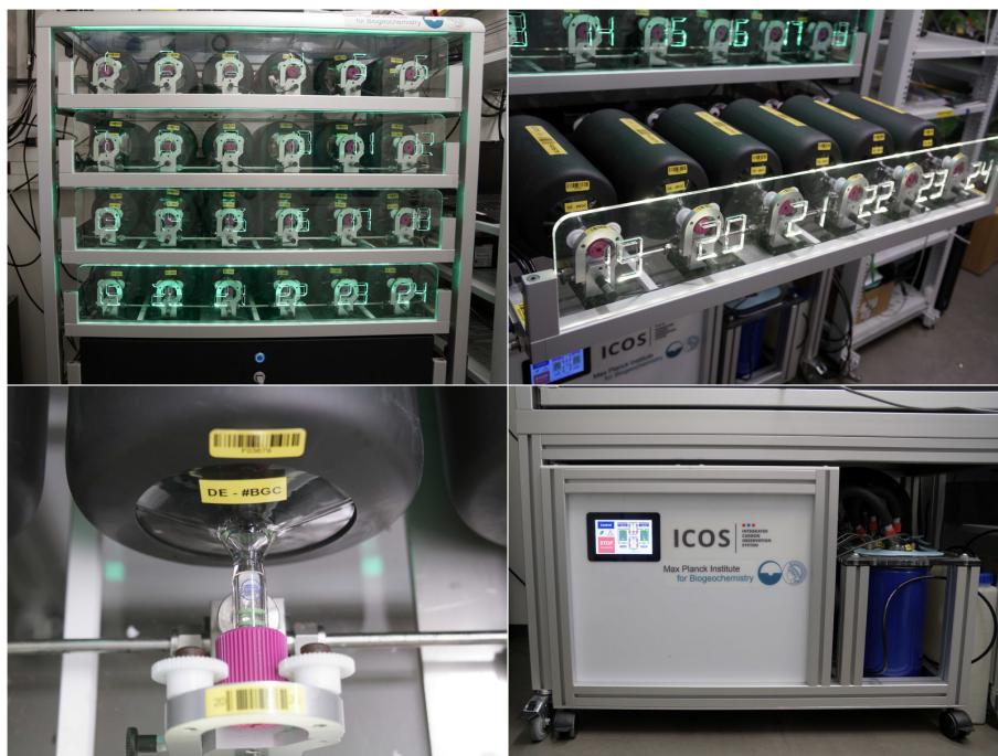
Figure 1. Automated flask sampler installed at the ATTO site. The sampler consists of four trays, and each tray holds six flasks, for a total of 24 flasks available for sampling. A drawer below the last tray contains all the electronic components and the compressor pump. The flasks are of 3 liter volume and samples are stored at an overpressure of \sim 0.7 bar. A drying unit (bottom right) takes the air drawn in by the sampler and cools it to a dew point below -38^{\circ}\text{C} .
