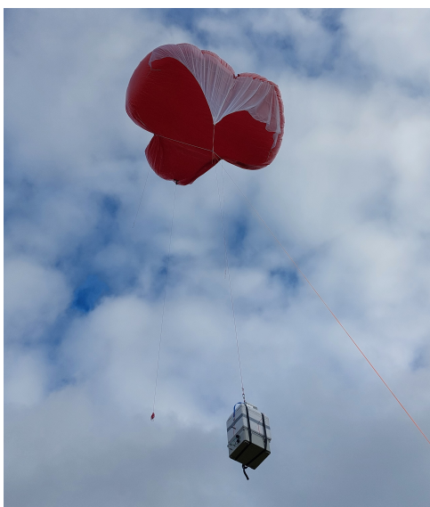
Figure 3. FMI's payload onboard onboard FMI's tethered balloon system Aerostat (SkyDoc Systems Inc.)
