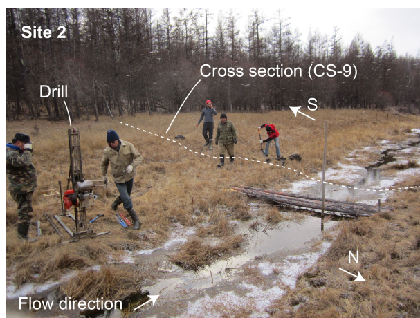
Figure D2. Installation of HOBO thermistor chains, and piezometer tubes at Site 2 (CS-9) with a petrol powered standing drill.
